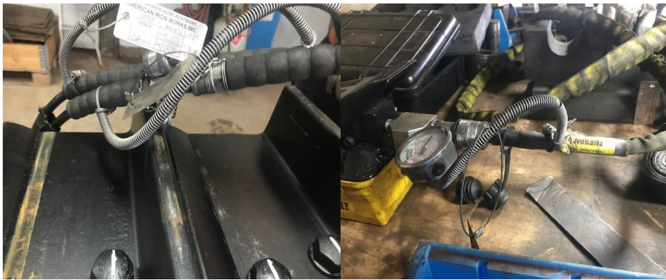
Figure 2: Certified high-pressure whip cords/hose chokers are used on all coupling connections.
