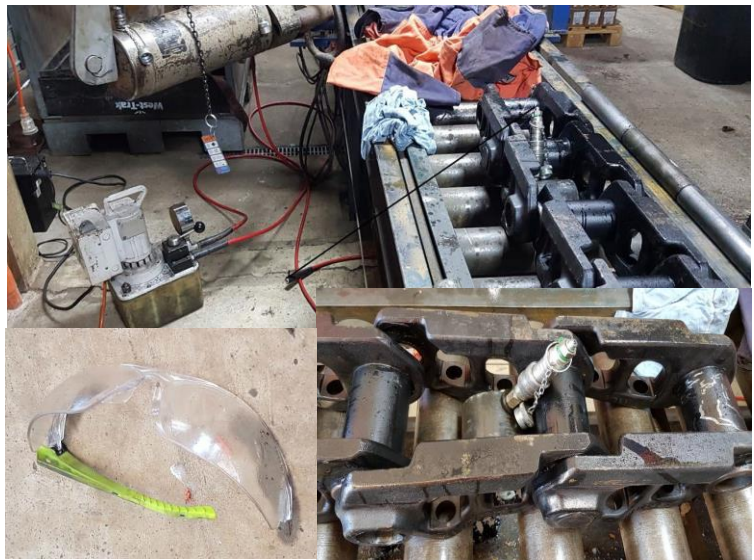
Figure 1: Hydraulic pump and hydraulic ram, with the failure occurring at the crimp of the hose tail. The safety glasses were found 3 meters from the operator, broken at the hinge
