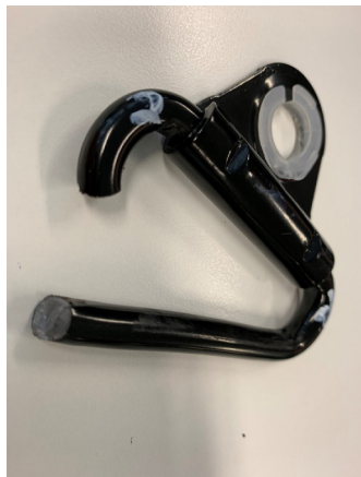
In crash testing, failure occurred in the shoulder anchor point (D-ring) and the retractor mechanism failed to lock and prevent runout of the belt.
