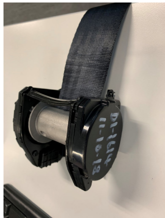
In crash testing, failure occurred in the shoulder anchor point (D-ring) and the retractor mechanism failed to lock and prevent runout of the belt.
