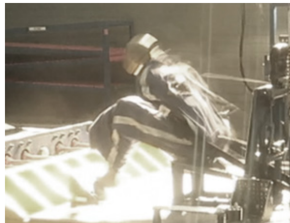
In the 50km/h test, the mannequin flies forward after the seatbelt fails.
