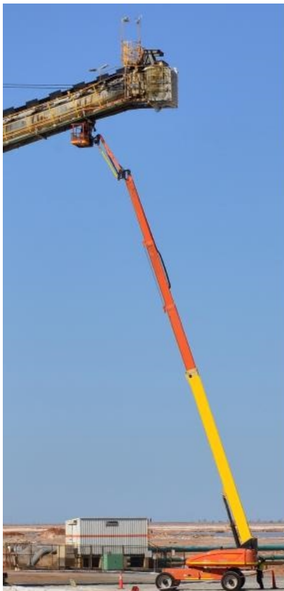
Elevating work platform operator trapped against underside of conveyor structure
