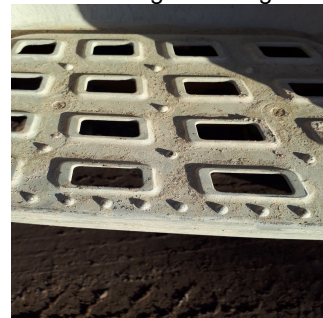
Footplate in good condition
