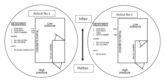
Airlock 1 (see image 1) is the design of the airlock the ERZ Controller was trapped in at the outbye door.
