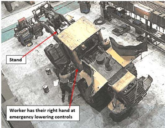
A maintenance worker was operating a ground controlled after-market manual emergency lowering system, to lower the boom of the IT onto a stand, when the front wheels lifted off the ground and the whole machine tilted over towards the worker.
