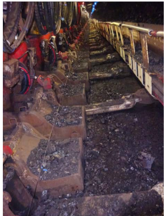
Figure 2: Ejected coal in the walkway as a result of the coal burst. ii
