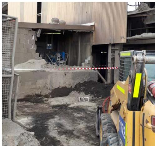
Spills should be eliminated as far as is reasonably practicable. In areas where spills cannot be avoided, the area should be designed to allow for safe cleaning and removal of material. The risk of falling material must also be controlled.
