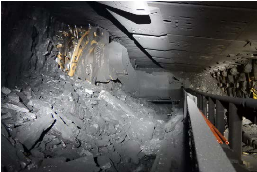
Figure 1: Maingate view of gas outburst. Supplied by Metropolitan Colliery.
