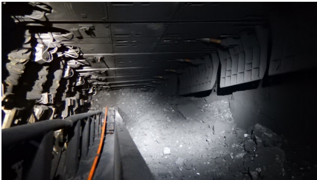
Figure 2: Tailgate view of gas outburst. Supplied by Metropolitan Colliery.
