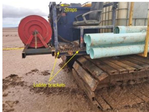
Cab of tracked vehicle. Note the straps used to hold control levers in place and the absence of the ladder (and position of brackets for ladder).
