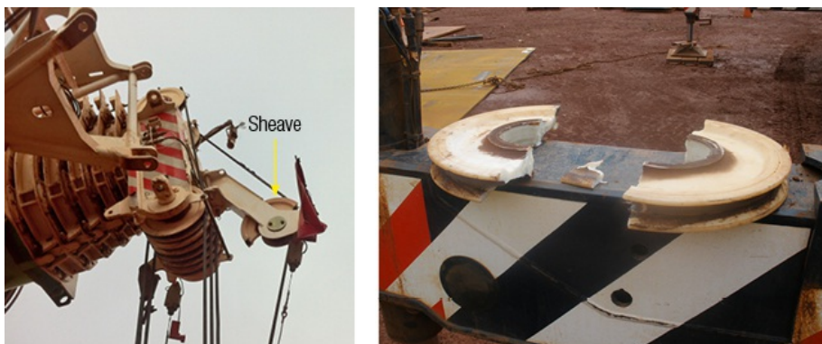
Damage to nylon head sheave. Right. Half of the failed sheave for the auxiliary hook remained in place. Left. Sheave sections recovered after the incident.
