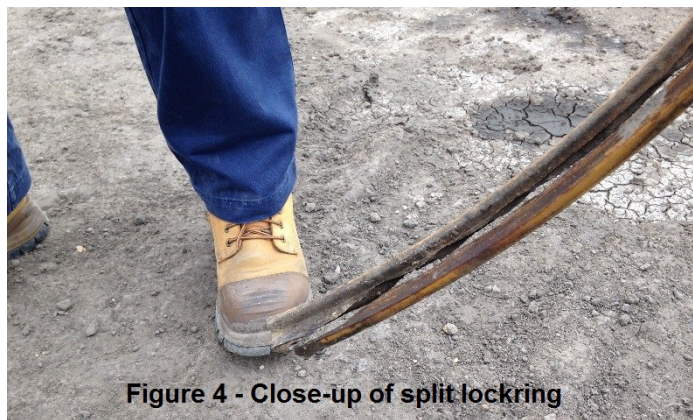
Figure 3 - Lockring: split circumferentially
