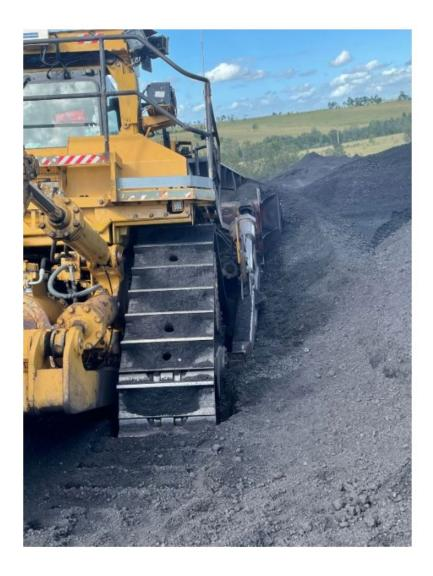
Comments to industry: The hazard of concealed voids exists on stockpiles and must be included in risk assessments, training and procedures for operators. Operators must be trained to identify when the risk of concealed voids is present and the procedure required to control the hazard.
